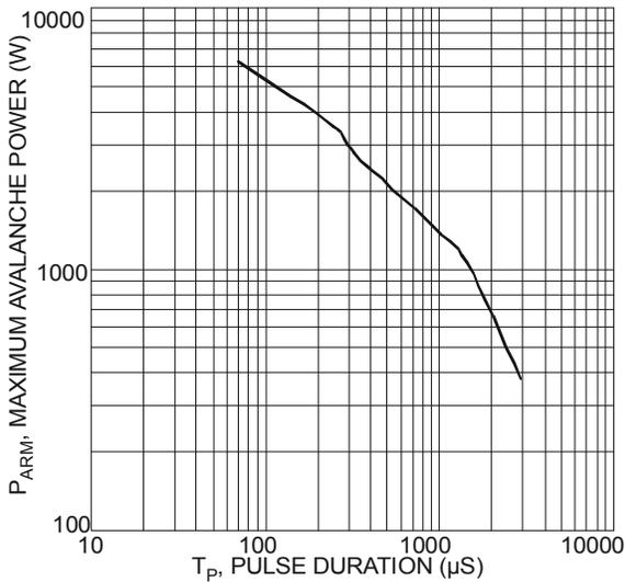
Figure 5 Maximum Avalanche Power Curve, Per Element
