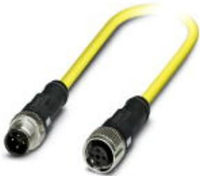
Sensor/Actuator cable, 4-position, PVC, yellow RAL 1021, Plug straight M12 SPEEDCON, A-coded, on Socket straight M12 SPEEDCON, A-coded, Cable length: 5 m
