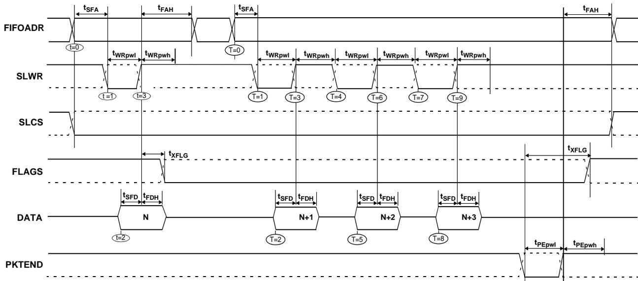
Figure 35 shows the timing relationship of the SLAVE FIFO write in an asynchronous mode. The diagram shows a single write followed by a burst write of 3 bytes and committing the 4byte short packet using PKTEND.
