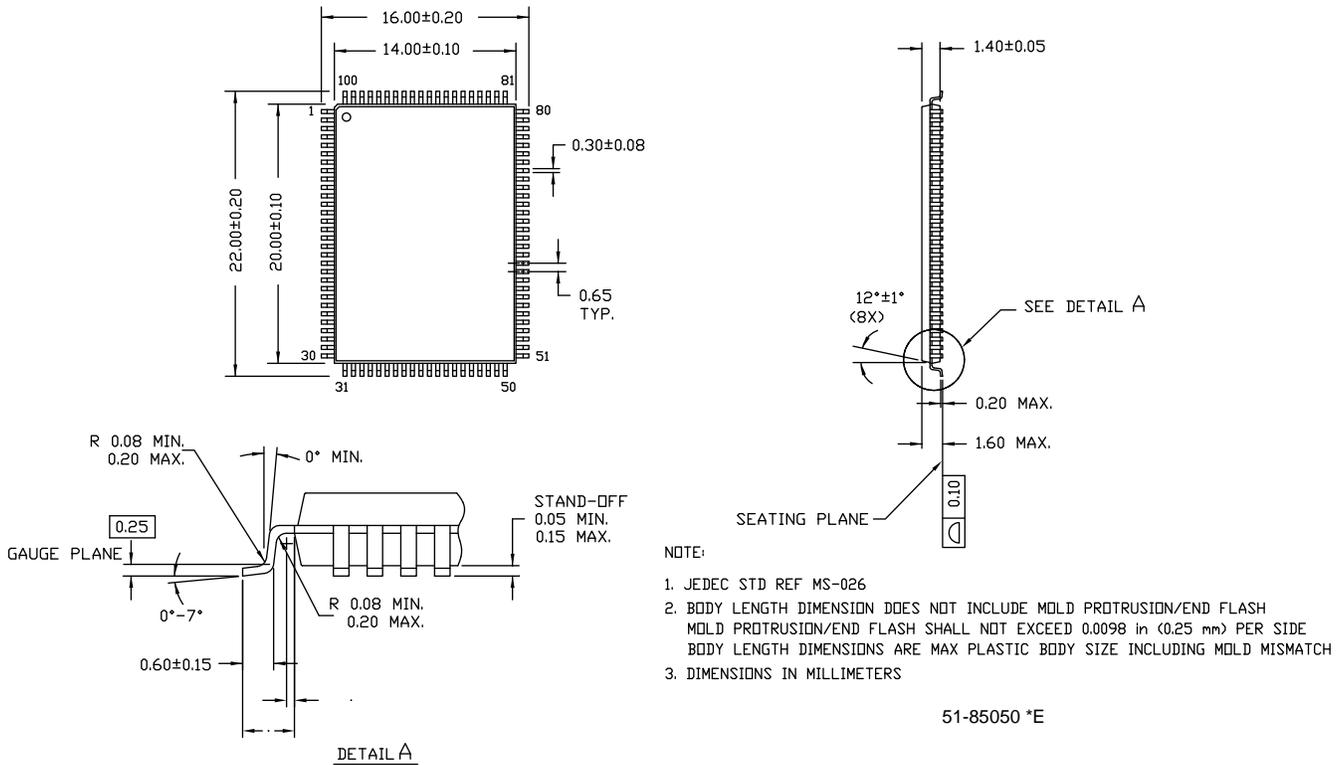
**Figure 39. 128-Pin Thin Plastic Quad Flatpack (14 x 20 x 1.4 mm) A128 (51-85101)**
