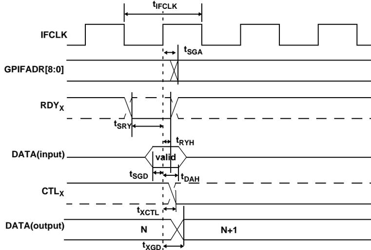
**Table 18. GPIF Synchronous Signals Parameters with Internally Sourced IFCLK<sup>[24, 25]</sup>**
