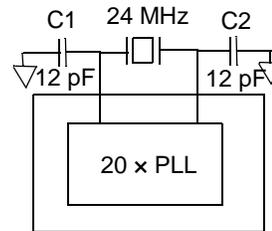
12-pF capacitor values assume a trace capacitance of 3 pF per side on a four-layer FR4 PCA
