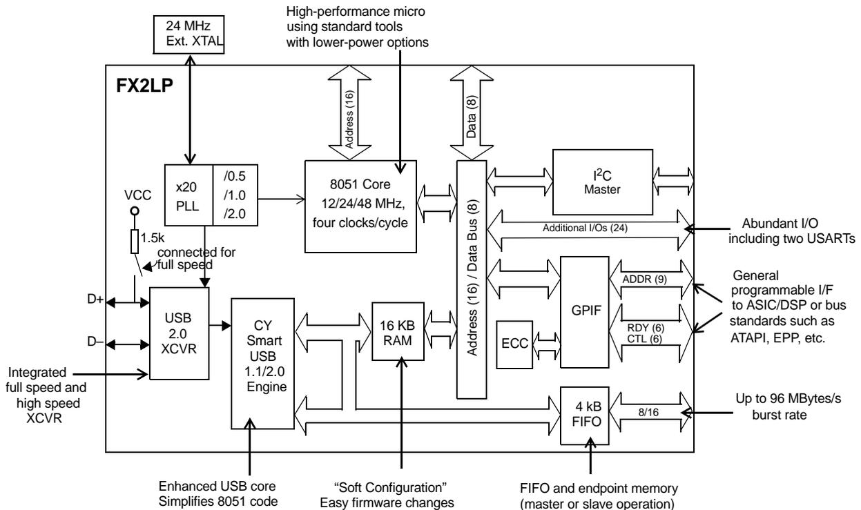
Cypress's EZ-USB® FX2LP™ (CY7C68013A/14A) is a low-power version of the EZ-USB FX2™ (CY7C68013), which is a highly integrated, low-power USB 2.0 microcontroller. By integrating the USB 2.0 transceiver, serial interface engine (SIE), enhanced 8051 microcontroller, and a programmable peripheral interface in a single chip, Cypress has created a cost-effective solution that provides superior time-to-market advantages with low power to enable bus-powered applications.
