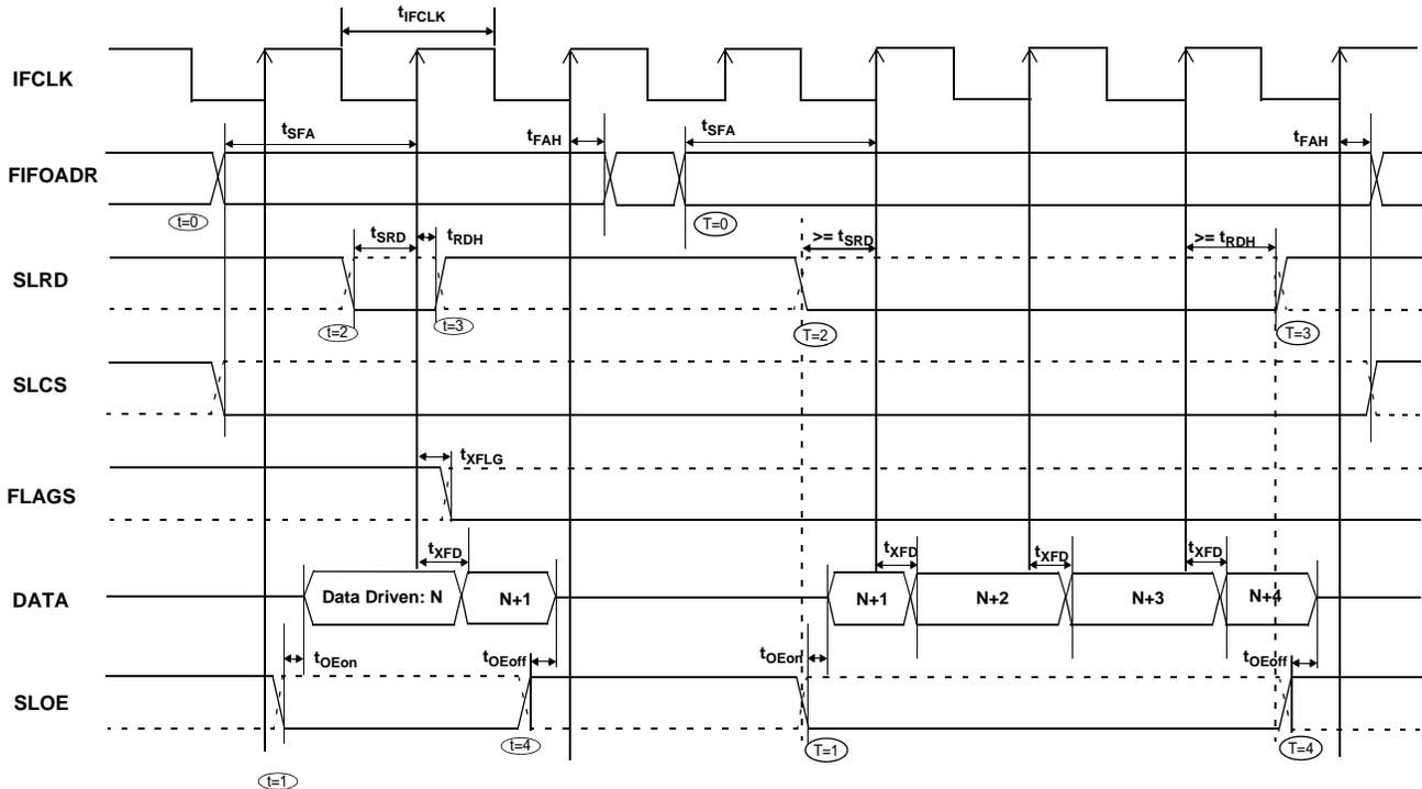
**Figure 31. Slave FIFO Synchronous Sequence of Events Diagram**
