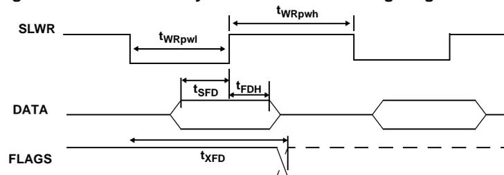
**Table 25. Slave FIFO Asynchronous Write Parameters with Internally Sourced IFCLK<sup>[27]</sup>**
