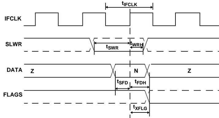
Table 23. Slave FIFO Synchronous Write Parameters with Internally Sourced IFCLK<sup>[25]</sup>
