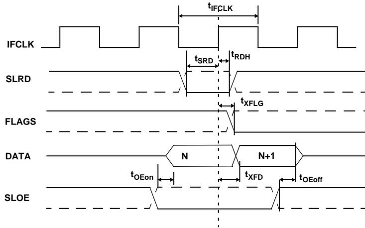
**Table 20. Slave FIFO Synchronous Read Parameters with Internally Sourced IFCLK<sup>[25]</sup>**
