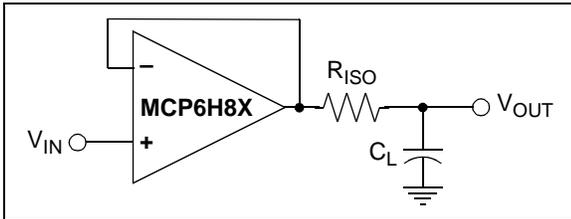
**FIGURE 4-4:** Output Resistor,  $R_{ISO}$  Stabilizes Large Capacitive Loads.
