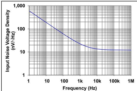
**FIGURE 2-8:** Input Noise Voltage Density vs. Frequency.
