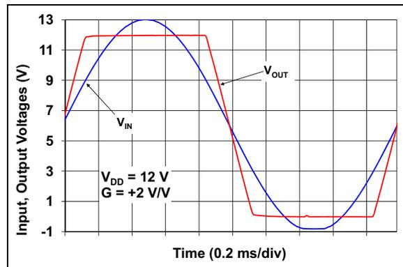
**FIGURE 2-36:** The MCP6H81/2/4 Shows No Phase Reversal.
