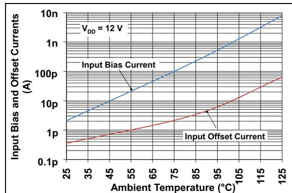
**FIGURE 2-12:** Input Bias, Offset Currents vs. Ambient Temperature.
