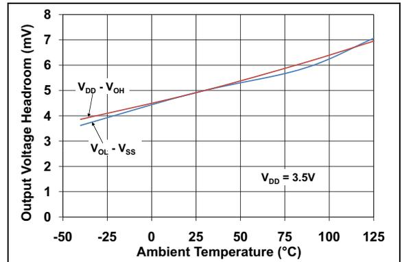
**FIGURE 2-29:** Output Voltage Headroom vs. Ambient Temperature.
