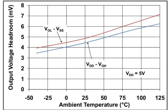
**FIGURE 2-28:** Output Voltage Headroom vs. Ambient Temperature.
