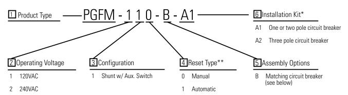
\*Note: Installation kits are for mounting the module and connecting to the tandem circuit breaker.
