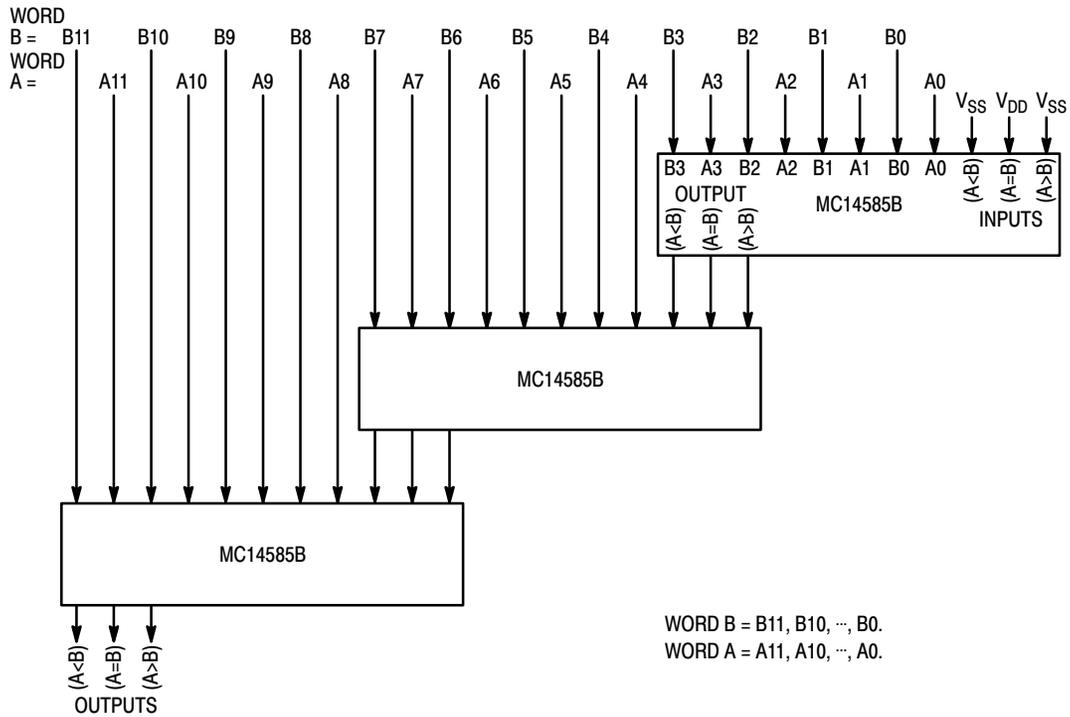
**Figure 3. Cascading Comparators**
