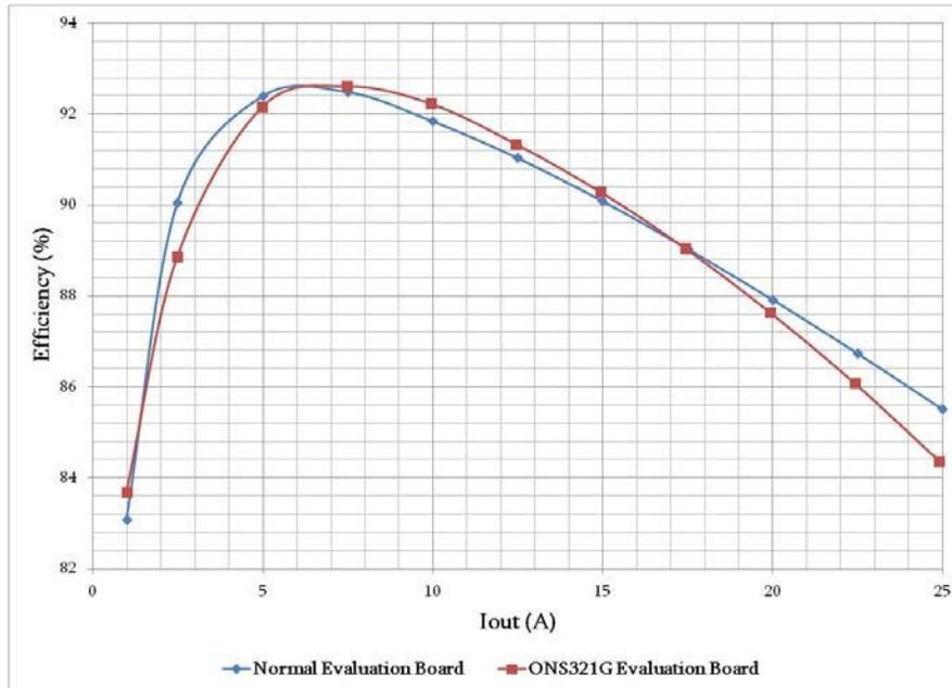
Figure 5. Comparison of Efficiency for Standard In-house and ONS321G Boards
