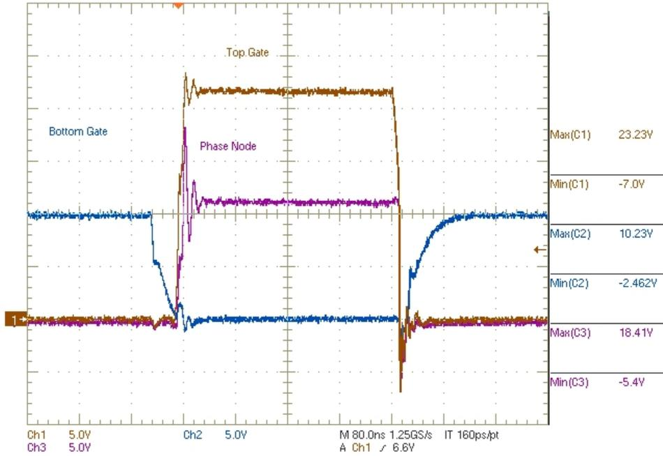
Figure 10. Switch Node Waveforms for  $V_{drvr} = 10\text{ V}$
