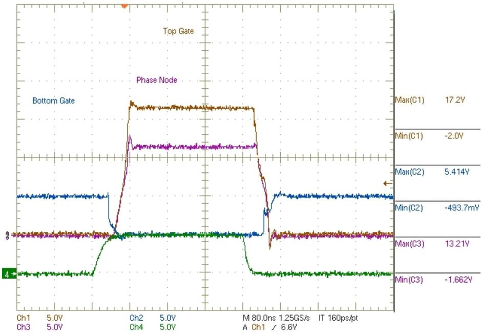
Figure 11. PWM Signal at G1 for  $I_{out} = 0\text{ A}$
