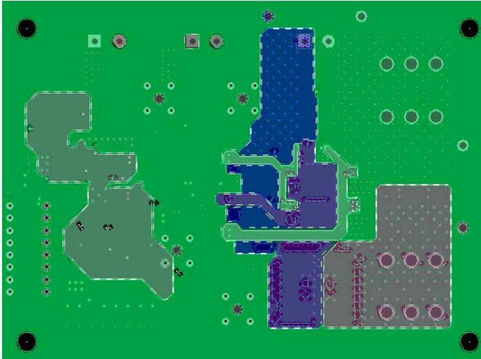
Figure 16. Internal Copper Layer 2 of ONS321G Evaluation Board
