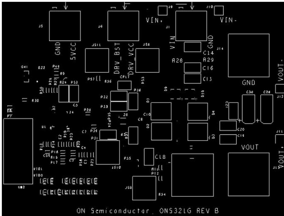
Figure 13. Top View of the ONS321G Evaluation Board
