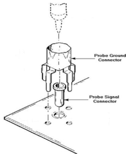
Figure 3. Tektronix Test Point & Probe Socket
