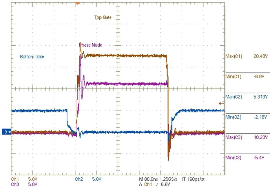
Figure 9. Switch Node Waveforms for  $V_{drvr} = 5\text{ V}$
