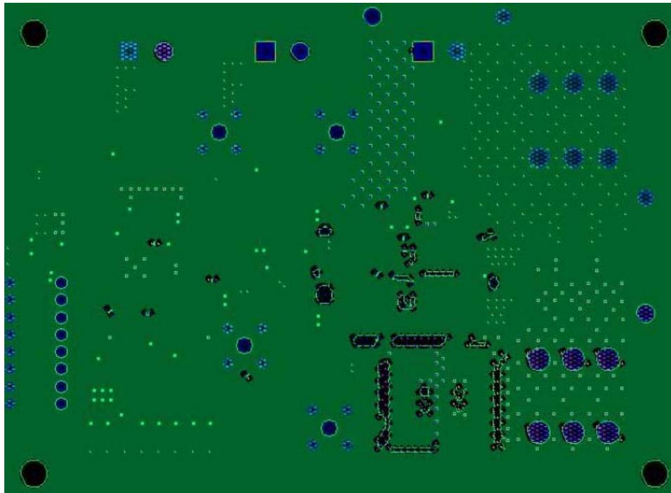
Figure 17. Internal Copper Layer 3 of ONS321G Evaluation Board
