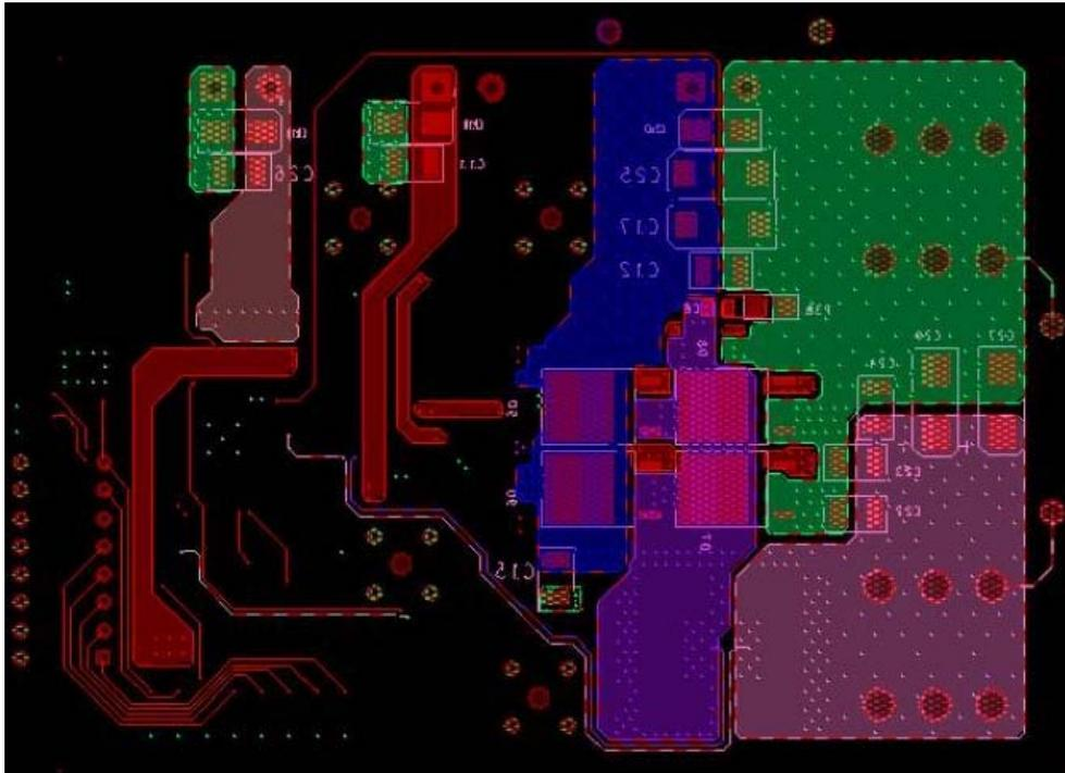
Figure 18. Copper Layer on the Bottom of ONS321G Evaluation Board
