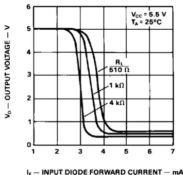
**Figure 3 Input Diode Forward Characteristics**
