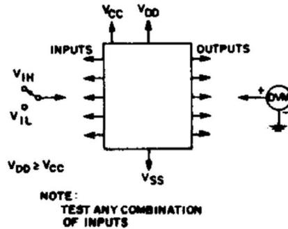
Figure 13. Input Voltage Test Circuit
