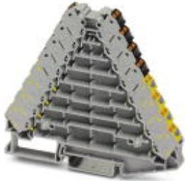
Potential distributors, Nom. voltage: 250 V, Nominal current: 17.5 A, Cross section: 0.14 mm<sup>2</sup> - 2.5 mm<sup>2</sup>, AWG: 14 - 26, Connection type: Push-in connection, Width: 8.3 mm, Length: 100 mm, Color: gray, Assembly: NS 35/7,5, NS 35/15
