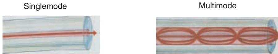
Multimode fiber was the first type of fiber to be commercialized. It has a much larger core than singlemode fiber, allowing hundreds of modes of light to propagate through the fiber simultaneously. Additionally, the larger core diameter of multimode fiber facilitates the use of lower-cost optical transmitters (such as light emitting diodes [LEDs] or vertical cavity surface emitting lasers [VCSELs]) and connectors.
