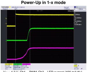
$V_{IN} = 4.2 V, Ch1 - PWM, Ch2 - LED current (400 mA/div), Ch3 - Output voltage$
