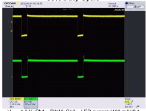
V<sub>IN</sub> = 4.2 V, Ch1 – PWM, Ch2 – LED current (400 mA/div)
