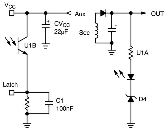
**Figure 25. You can either directly observe the  $V_{CC}$  level or add a small RC filter to reduce the leakage inductance contribution. The best is to directly sense the output voltage and reacts if it runs away, as offered on the right side.**
