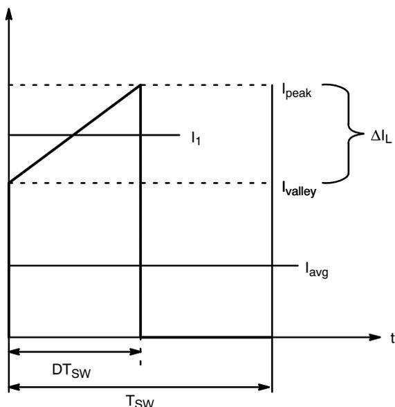
**Figure 26. Primary Inductance Current Evolution in CCM**
