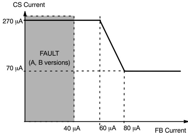
**Figure 16. The NCP1351 Peak Current Compression Scheme**
