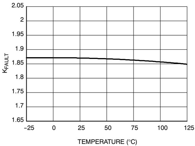
**Figure 41. K\_FAULT Variations versus Junction Temperature**
