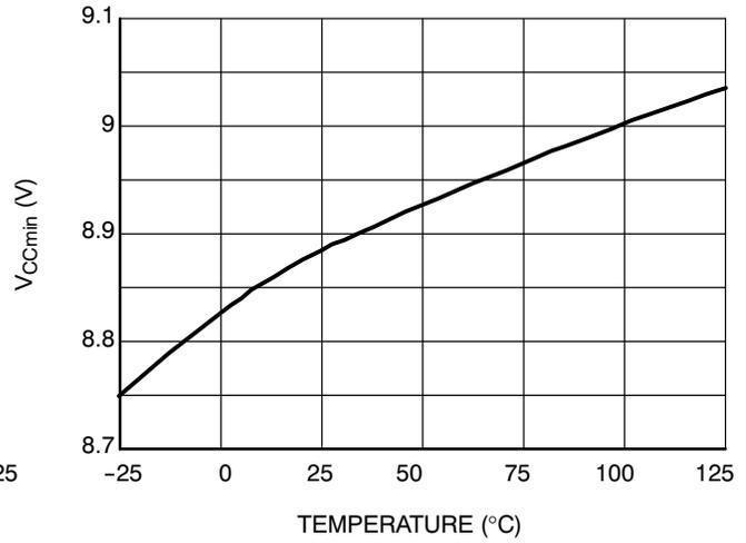
**Figure 34. V<sub>CCmin</sub> Level versus Junction Temperature**
