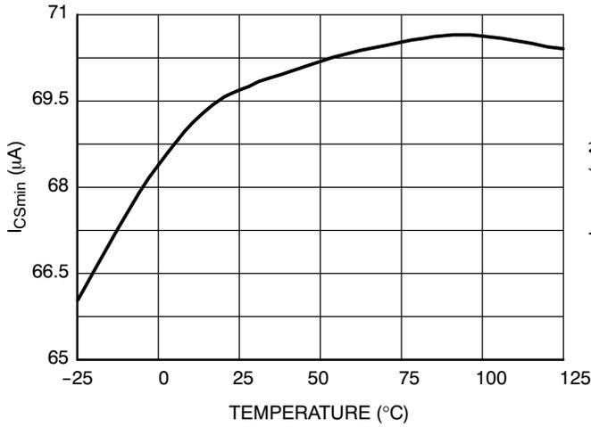
**Figure 35. I<sub>CSmin</sub> versus Junction Temperature**
