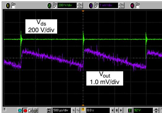
**Figure 29. No-Load Output Ripple**
