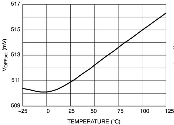
**Figure 37. Oscillator Offset Voltage versus Junction Temperature**
