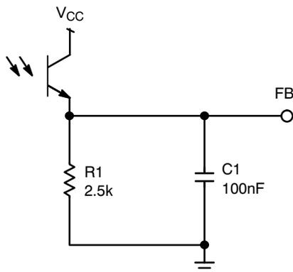
**Figure 17. The Recommended Feedback Arrangement Around the FB Pin**
