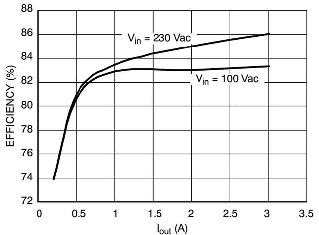
Figure 28. Efficiency Measured at Various Operating Points
