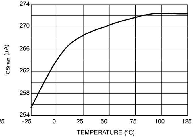
**Figure 36. I<sub>CSmax</sub> versus Junction Temperature**
