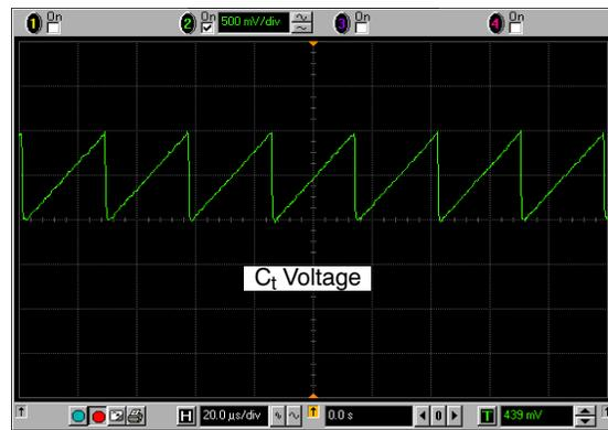
Figure 12.  $C_t$  Voltage Swing at a Moderate Loading
