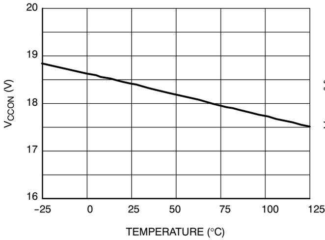
**Figure 33. V<sub>CCON</sub> Level versus Junction Temperature**
