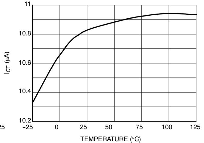
**Figure 38. Timing Capacitor Charge-Current Variation versus Junction Temperature**
