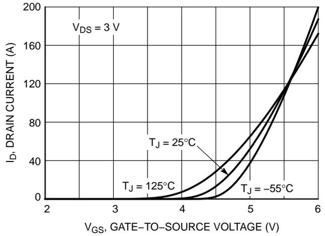
Figure 2. Transfer Characteristics
