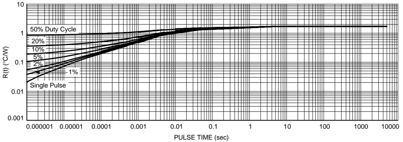
Figure 13. Thermal Characteristics
