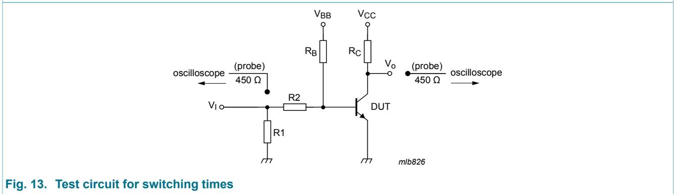
Fig. 13. Test circuit for switching times
