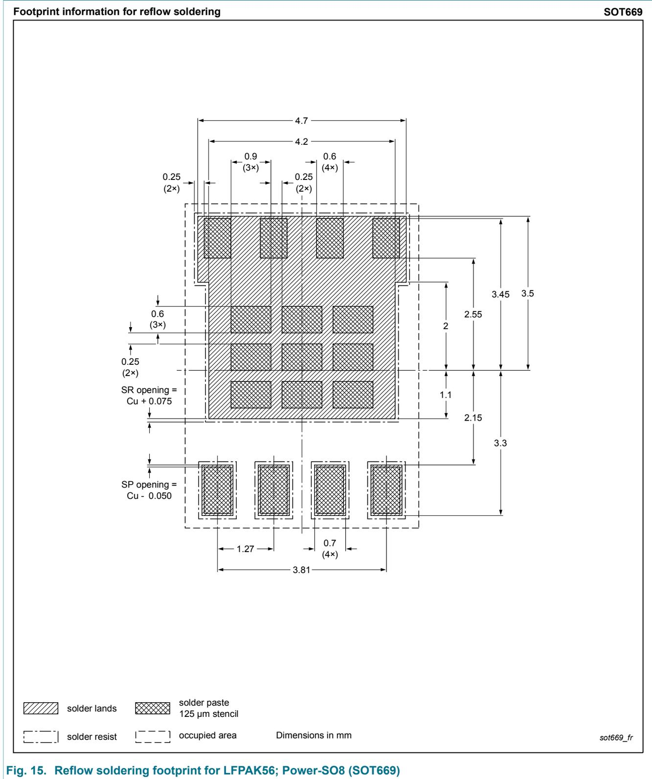
Fig. 15. Reflow soldering footprint for LPAK56; Power-SO8 (SOT669)
