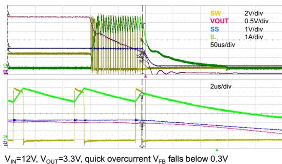
Figure 18. Start-up with shorted  $V_{OUT}$
