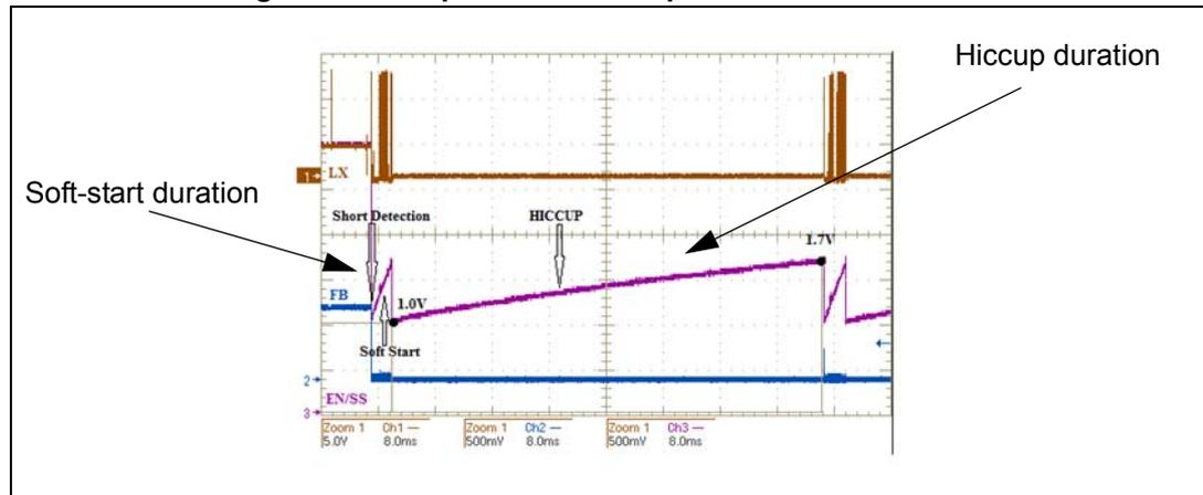
The HICCUP time depends on the selected value of the soft-start capacitor, considering  $R_{SS} = 4.7 \text{ M}\Omega$  fixed value (see [Section 6.5 on page 19](#)).
