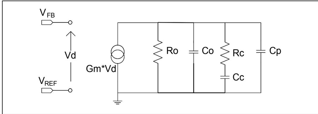
$R_C$  and  $C_C$  are the compensation network,  $R_O$  represents output resistance of the error amplifier,  $C_o$  represents the internal low frequency pole of the error amplifier.
