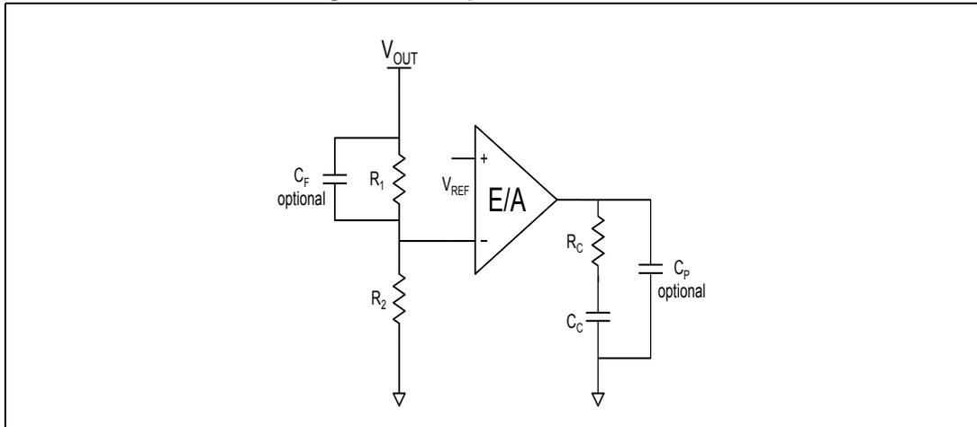
Starting from the target bandwidth ( $f_{BW}$ ) the compensation network values can be calculated to have a stable loop response basing [Equation 22](#) and [Equation 23](#).
