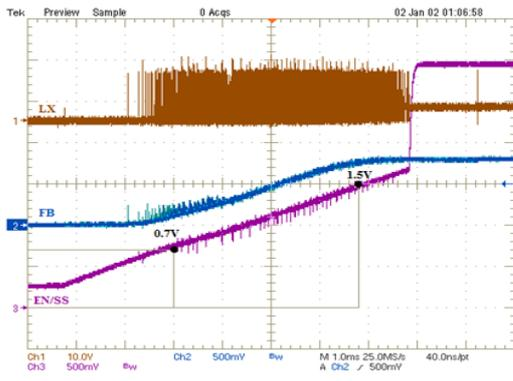
Figure 16. Long overload condition
