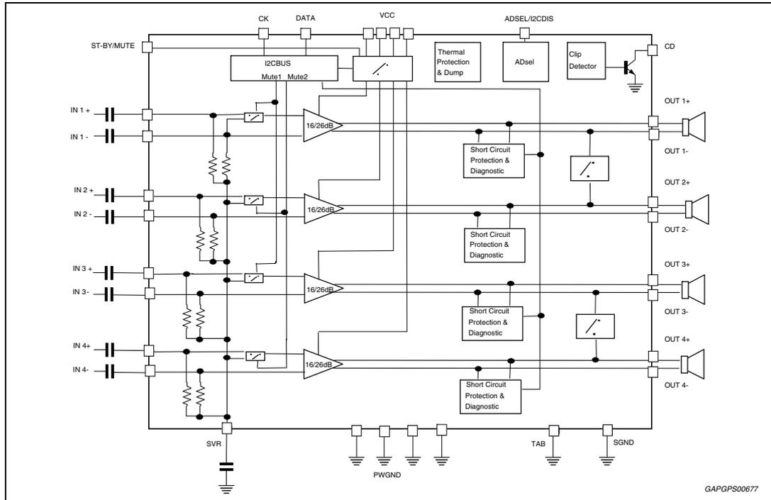
Figure 2. Application circuit
