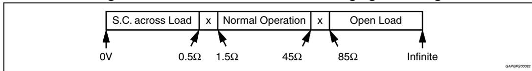
If the Line-Driver mode (Gv= 16 dB and Line Driver Mode diagnostic = 1) is selected, the same thresholds will change as follows:
