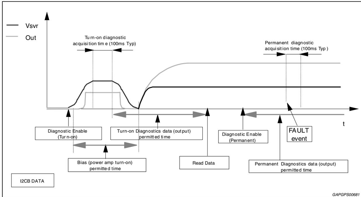
The information related to the outputs status is read and memorized at the end of the current pulse top. The acquisition time is 100 ms (typ.). No audible noise is generated in the process. As for SHORT TO GND / Vs the fault-detection thresholds remain unchanged from 26 dB to 16 dB gain setting. They are as follows: TDA75610DLVPD
