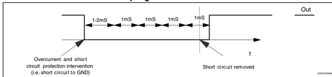
**Figure 29. Restart timing with diagnostic enable (permanent)**
