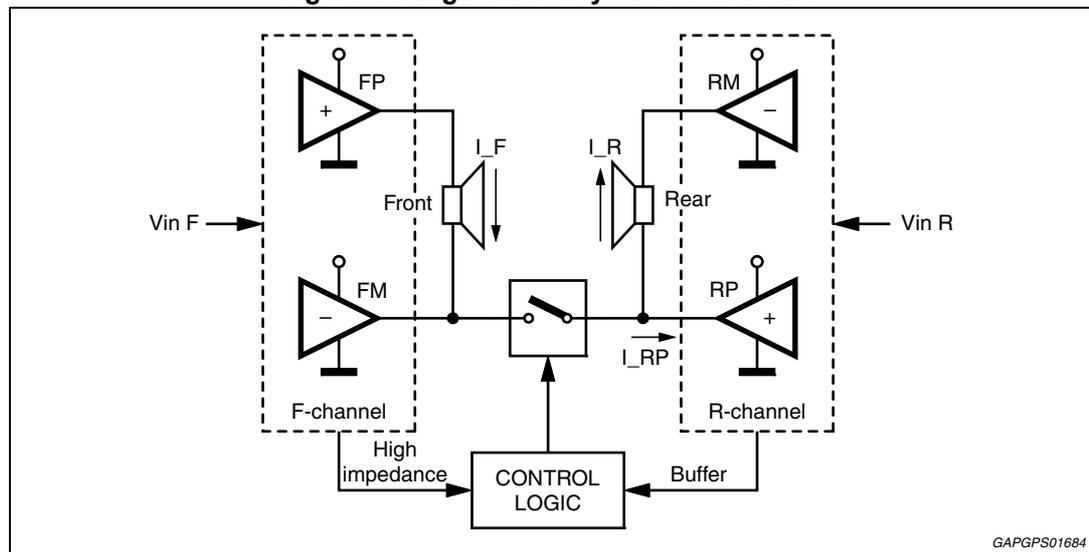
When the power demand increases to more than 2.5 W, the system behavior is switched back to a standard double bridge in order to guarantee the maximum output power, while in the 6 V start-stop devices the High Efficiency mode is automatically disabled at low  $V_{CC}$  ( $7.3\text{ V} \pm 0.3\text{ V}$ ). No need to re-program it when  $V_{CC}$  goes back to normal levels.
