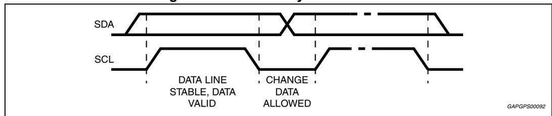
**Figure 38. Timing diagram on the I<sup>2</sup>C bus**
