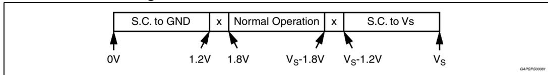
Concerning SHORT ACROSS THE SPEAKER / OPEN SPEAKER, the threshold varies from 26 dB to 16 dB gain setting, since different loads are expected (either normal speaker's impedance or high impedance). The values in case of 26 dB gain are as follows:
