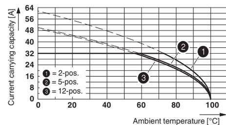
Derating curve for: DFK-PC 5/...-ST-7,62 with PC 5/...-ST-7,62
