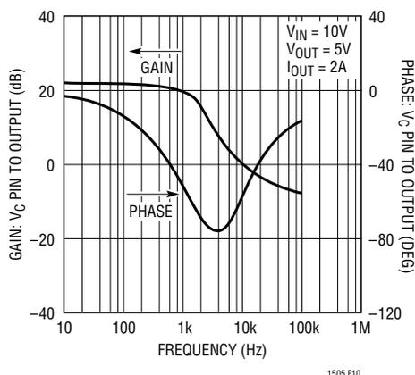
Figure 10. Response from  $V_C$  Pin to Output
