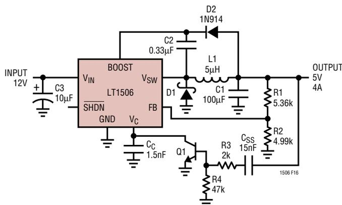
Figure 16. Buck Converter with Adjustable Soft Start
