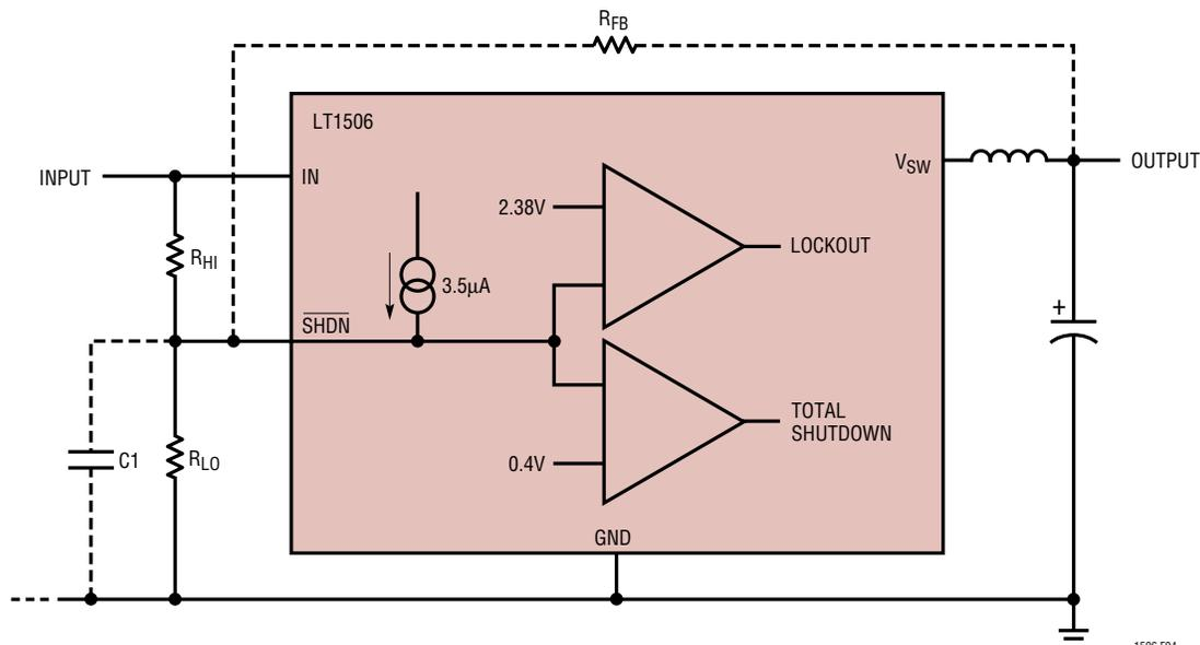
**Figure 4. Undervoltage Lockout**
