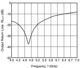
ANT1-RX OUTPUT RETURN LOSS vs. FREQUENCY (When ANT1-RX is ON)
