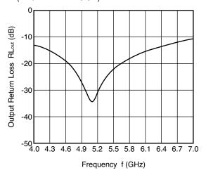
TX-ANT2 OUTPUT RETURN LOSS vs. FREQUENCY (When TX-ANT2 is ON)
