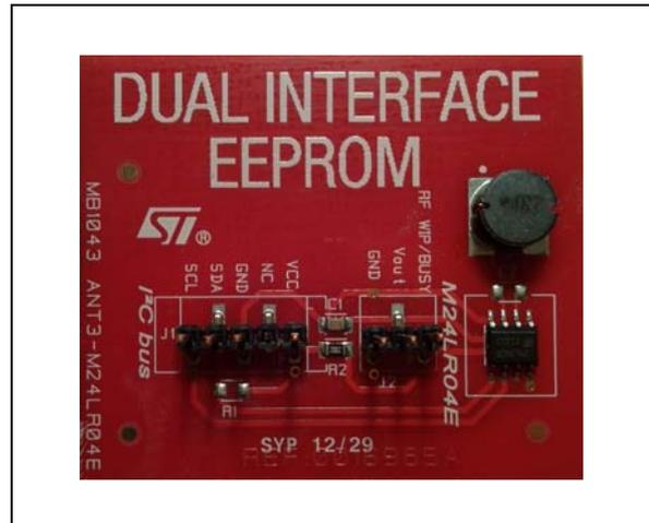
The ANT3-M24LR04E antenna allows system designers to evaluate the M24LR04E-R performance and capabilities, and to get started with their design.
