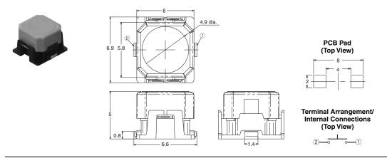
$\textbf{Note:} \quad \text{Unless otherwise specified, a tolerance of $\pm 0.4$ mm applies to all dimensions. No terminal numbers are indicated on the Switches.}$
