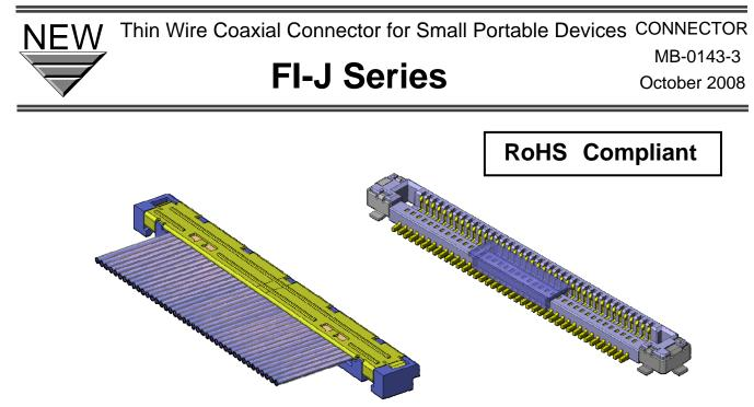
The FI-J Series is a thin-wire coaxial connector compatible with 42 and 44 AWG wires, and it is ideally suited for compact devices. The FI-J achieves remarkable space saving on the board and is small enough to pass through a narrow hinge after the harness is assembled.
