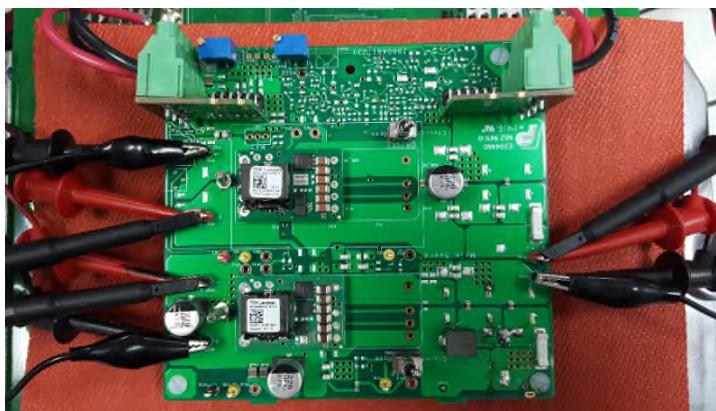
Be aware that the loop formed by the scope probe's ground lead may pick up spurious switching noise.
