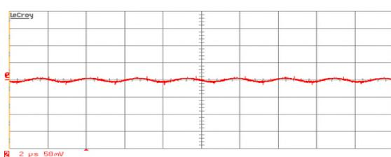
Full load output ripple with scope socket
