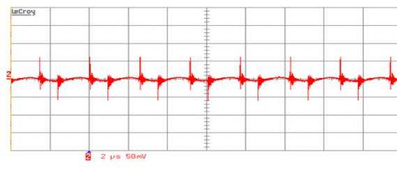
Full load output ripple with ground loop acting as an antenna
