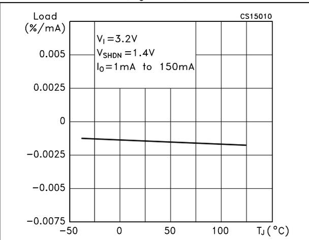
Figure 14. Load regulation vs. temperature ( $V_0=3.3\text{ V}$ )
