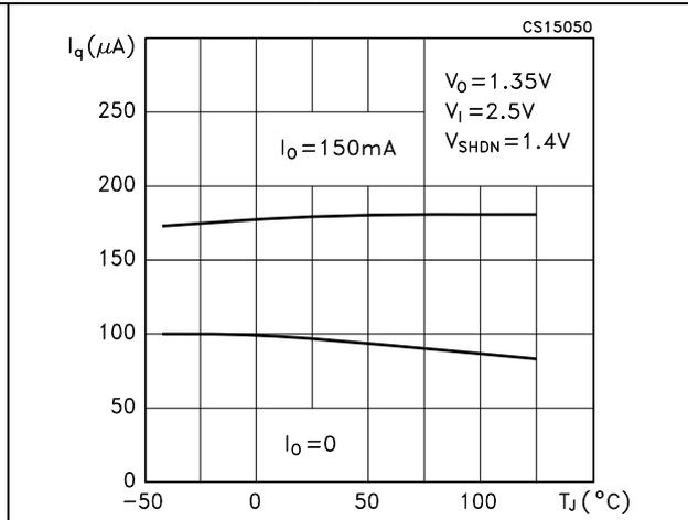
Figure 16. Quiescent current vs. temperature ( $V_I=6\text{ V}$ )
