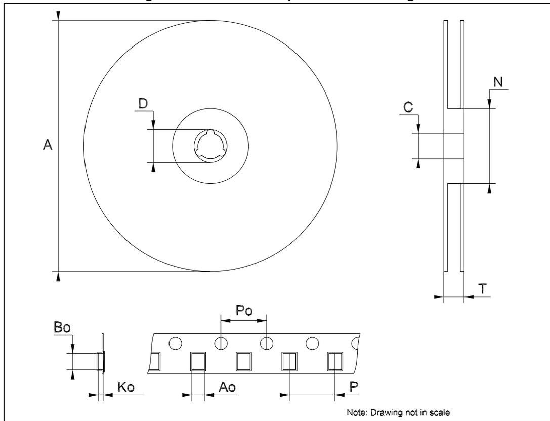
Table 9. Flip-chip 5 tape and reel mechanical data
