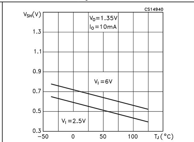
Figure 8. Shutdown voltage vs. temperature
