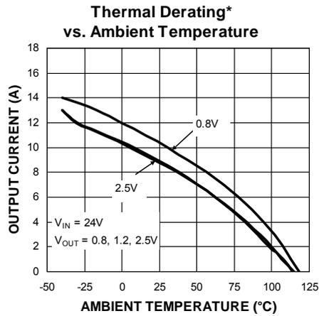
**Die Temperature\*** : The temperature measurement was taken at the hottest point on the MIC261201 case mounted on a 5 square inch 4 layer, 0.62", FR-4 PCB with 2oz finish copper weight per layer, see Thermal Measurement section. Actual results will depend upon the size of the PCB, ambient temperature and proximity to other heat emitting components.
