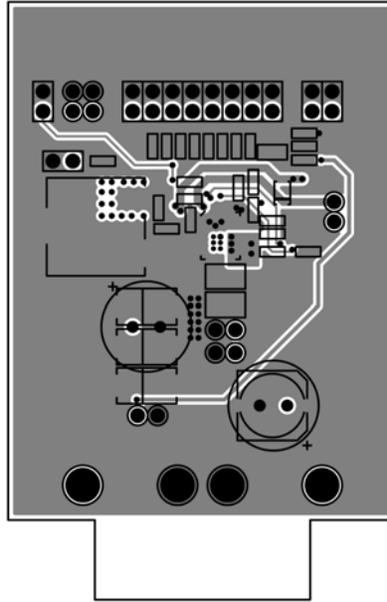
Figure 11. MIC261201 Evaluation Board Mid-Layer 2
