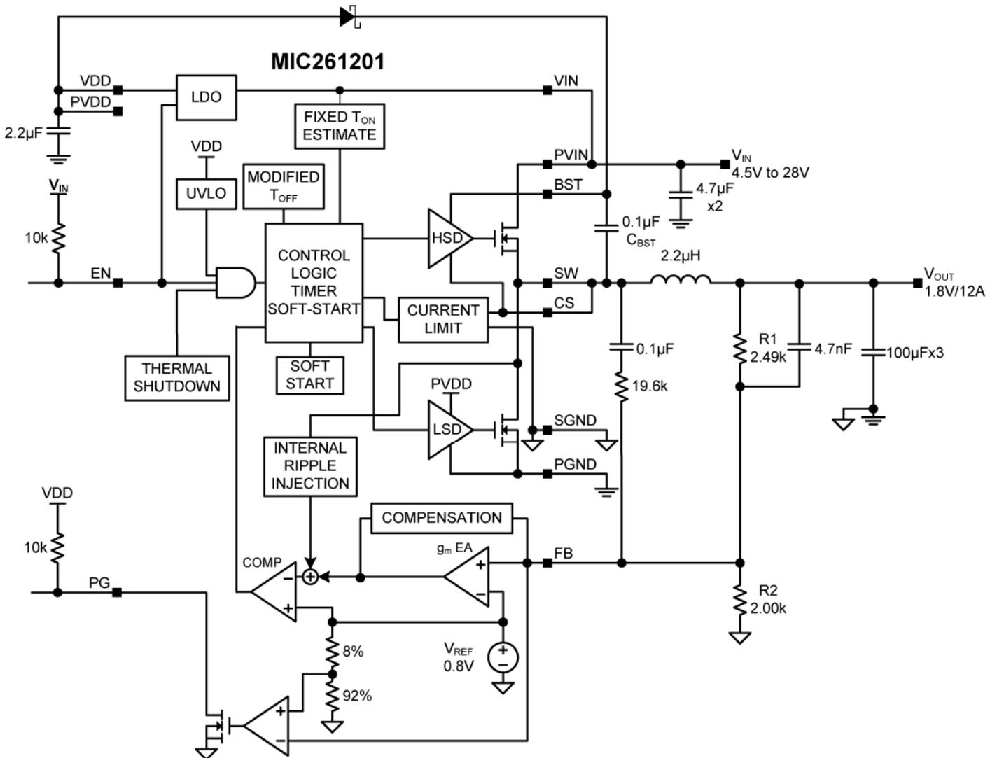
Figure 1. MIC261201 Block Diagram
