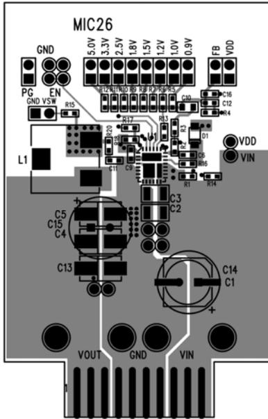
Figure 9. MIC261201 Evaluation Board Top Layer
