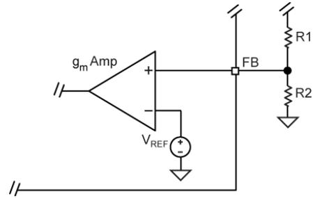
Figure 6. Voltage-Divider Configuration
