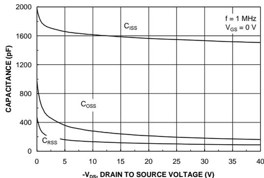
Figure 18. Capacitance Characteristics.
