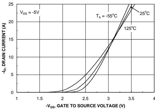
Figure 15. Transfer Characteristics.
