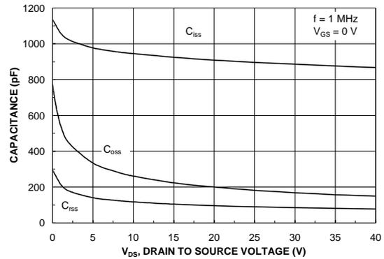
Figure 8. Capacitance Characteristics.
