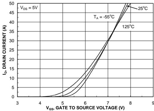
Figure 5. Transfer Characteristics.
