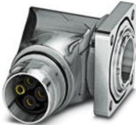
Device connector, front mounting, angled rotatable, SPEEDCON locking, M17, Number of positions: 5+PE, Type of contact: Male connector, Crimp connection, Axial O-ring, 4xØ2,7, shielded: yes, Flange dimensions: 25.75 mm x 25.75 mm
