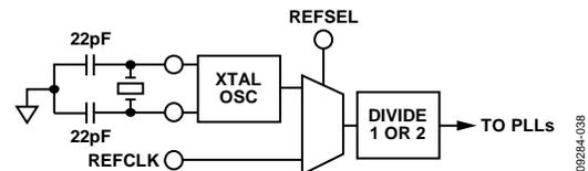
Figure 34. Reference Input Section and Reference Dividers
