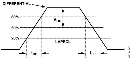
Figure 2. LVPECL Timing, Differential
