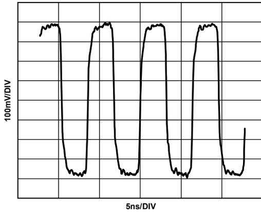
Figure 21. Typical LVDS Differential Output Trace, 156.25 MHz
