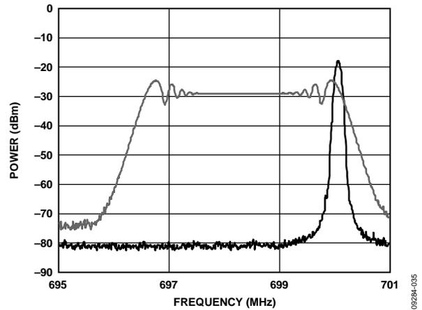
Figure 31. Typical Nonspread and Spread Spectrum Power Spectra, OUT2, Nb = 96, FRAC = 0, MOD = 1000, CkDiv = 7, NumSteps = 59, FracStep = -8, f<sub>OUT</sub> = 100 MHz with -0.5% Downspread at 30.2 kHz, MAX\_BW set to 0, Seventh Harmonic Shown, Spectrum Analyzer Resolution Bandwidth = 120 kHz, Maximum Hold On
