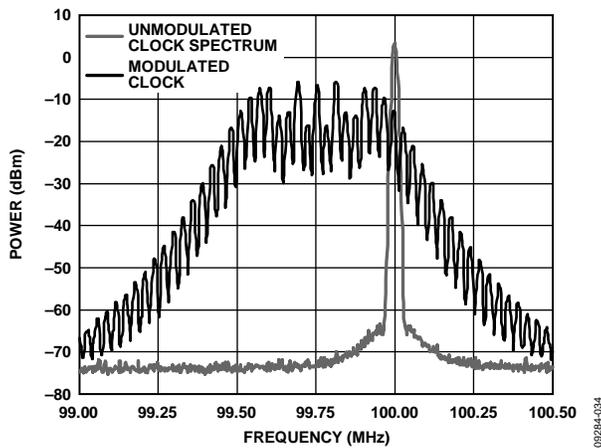
Figure 30. Typical Nonspread and Spread Spectrum Power Spectra, OUT2, Nb = 96, FRAC = 0, MOD = 1000, CkDiv = 7, NumSteps = 59, FracStep = -8, f<sub>OUT</sub> = 100 MHz with -0.5% Downspread at 30.2 kHz, MAX\_BW set to 0, First Harmonic Shown, Spectrum Analyzer Resolution Bandwidth = 10 kHz, Maximum Hold On
