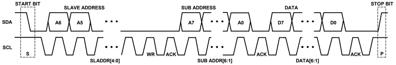
Figure 47. I<sup>2</sup>C Data Transfer Timing
