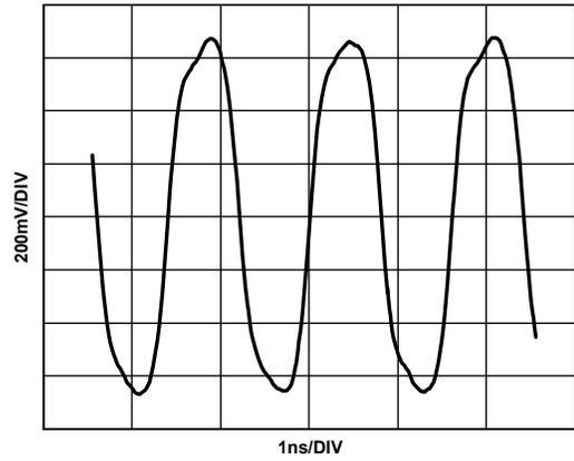
Figure 23. Typical LVPECL Differential Output Trace, 625 MHz
