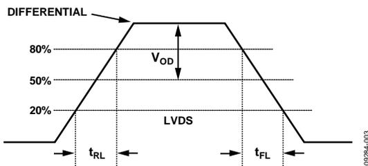
Figure 3. LVDS Timing, Differential
