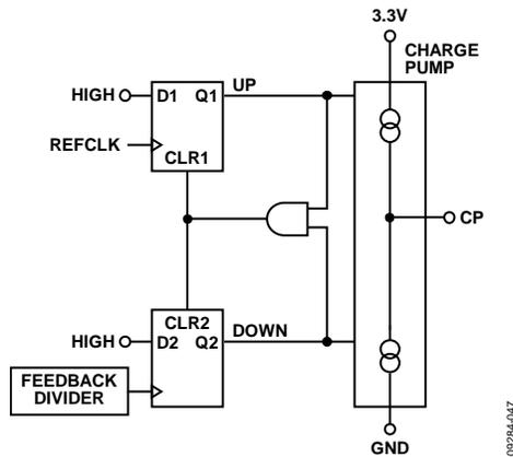
Figure 42. PFD Circuit Showing Simplified Charge Pump
