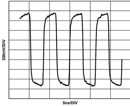
Figure 20 Typical LVPECL Differential Output Trace, 156.25 MHz
