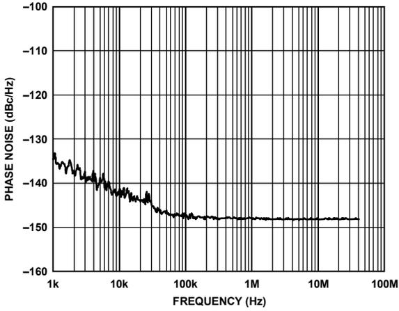
Figure 6. Phase Noise, REFOUT Output, 25 MHz ( $f_{XTAL} = 25$  MHz)
