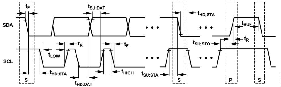
Figure 48. I<sup>2</sup>C Port Timing Diagram
