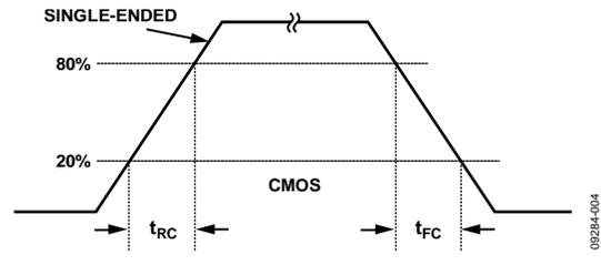
Figure 4. CMOS Timing, Single-Ended, 5 pF Load
