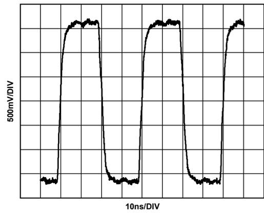
Figure 25. Typical REFOUT Output Trace, 25 MHz
