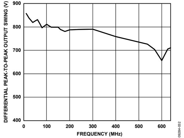
Figure 28. LVDS Differential, Peak-to-Peak Output Swing vs. Frequency
