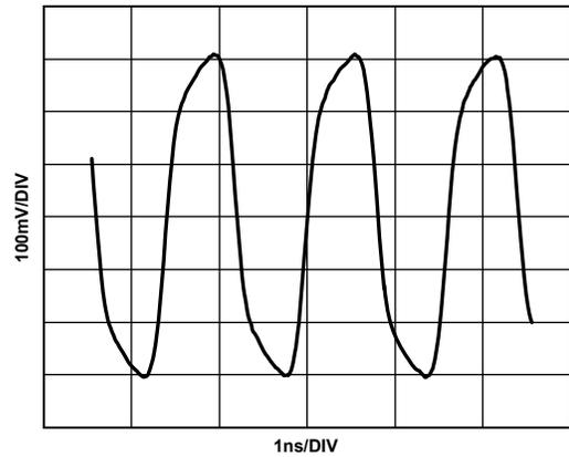
Figure 24. Typical LVDS Differential Output Trace, 625 MHz
