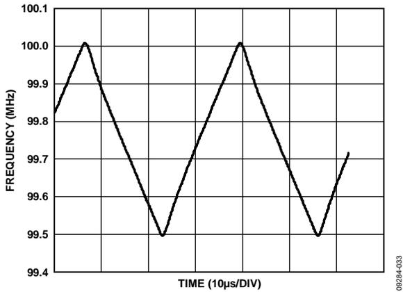
Figure 29. Typical Spread Spectrum Frequency Modulation Profile OUT2, Nb = 96, FRAC = 0, MOD = 1000, CkDiv = 7, NumSteps = 59, FracStep = -8, f<sub>OUT</sub> = 100 MHz with -0.5% Downspread at 30.2 kHz, MAX\_BW set to 0
