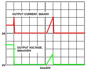
FIGURE 14. OVERCURRENT BEHAVIOR IN HICCUP MODE
