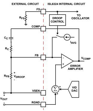
FIGURE 8. OUTPUT VOLTAGE AND LOAD-LINE REGULATION
