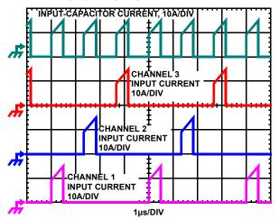
FIGURE 2. CHANNEL INPUT CURRENTS AND INPUT
