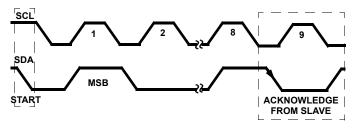
FIGURE 17. ACKNOWLEDGE ON THE I<sup>2</sup>C BUS
