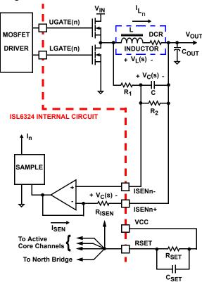
FIGURE 21. DCR SENSING CONFIGURATION
