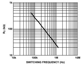
FIGURE 25. RT vs SWITCHING FREQUENCY
