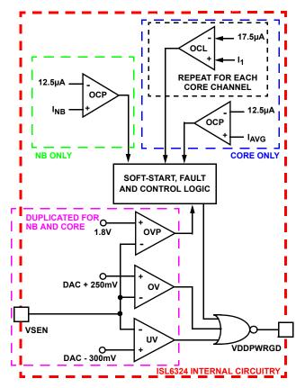
FIGURE 13. POWER-GOOD AND PROTECTION CIRCUITRY
