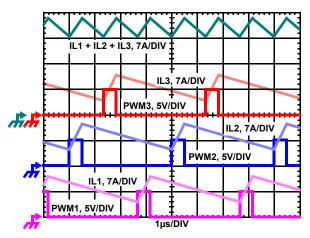
FIGURE 1. PWM AND INDUCTOR-CURRENT WAVEFORMS
