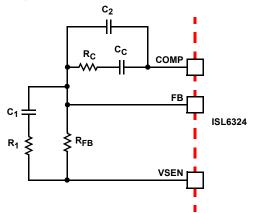
FIGURE 24. COMPENSATION CIRCUIT WITHOUT LOAD-LINE REGULATION
