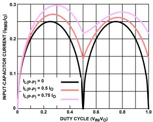
FIGURE 28. NORMALIZED INPUT-CAPACITOR RMS
