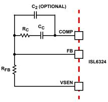
FIGURE 23. COMPENSATION CONFIGURATION FOR LOAD-LINE REGULATED ISL6324 CIRCUIT
