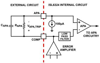
FIGURE 3. ADAPTIVE PHASE ALIGNMENT DETECTION
