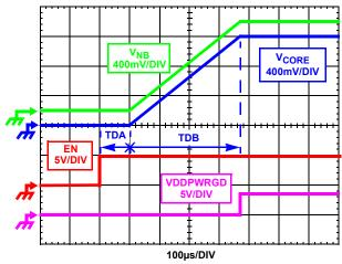
FIGURE 11. SOFT-START WAVEFORMS
