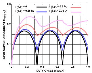
FIGURE 27. NORMALIZED INPUT-CAPACITOR RMS
