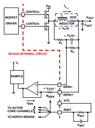
FIGURE 5. INDUCTOR DCR CURRENT SENSING CONFIGURATION
