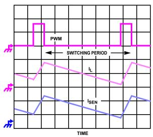
FIGURE 4. CONTINUOUS CURRENT SAMPLING
