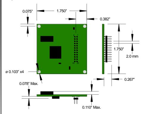
Connector: 24-Pin Header 0.5mm Square Pins 2.0mm Pin Spacing Samtec P# TMM-112-06-T-D-SM
