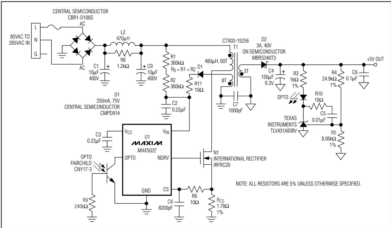
Figure 1. Universal 5W Off-Line Standby Power Supply
