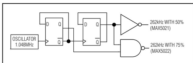
Figure 3. Internal Oscillator
