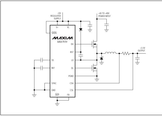
Figure 1. Powering V+ and VL from a Regulated +5V supply
