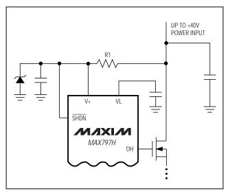
Figure 4. Powering V+ with a Zener Shunt Regulator
