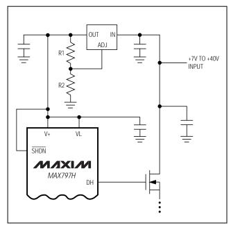
Figure 2. Powering V+ and VL with a +5V Linear Regulator
