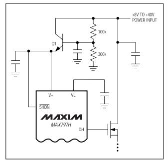
Figure 3. Dividing the Power Input to Supply V+
