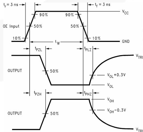
**Figure 6. AC Waveforms**
