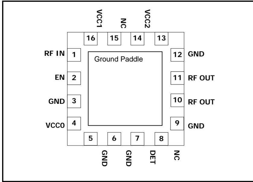
**Figure 2: SE2565T Pin Out (Top View Through Package)**
