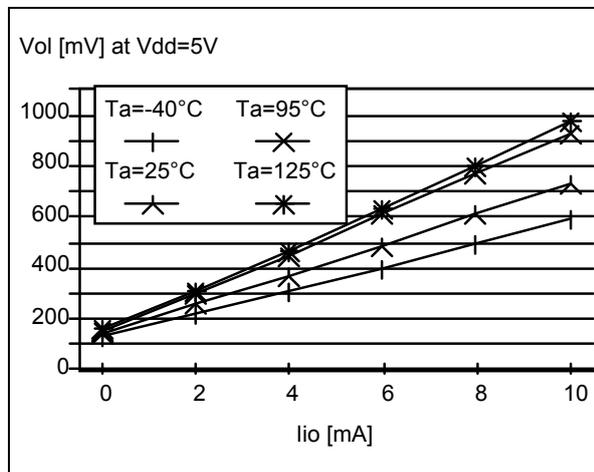
Figure 64. Typical  $V_{OL}$  at  $V_{DD} = 5V$  (high-sink)
