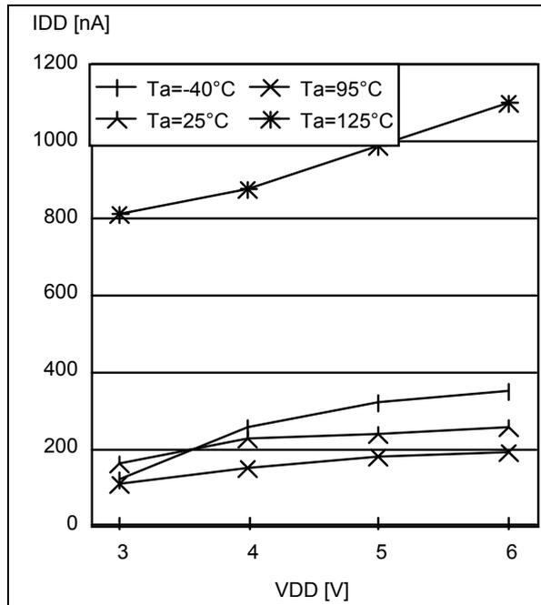
Figure 48. Typical I<sub>DD</sub> in STOP vs Temperature for ROM devices
