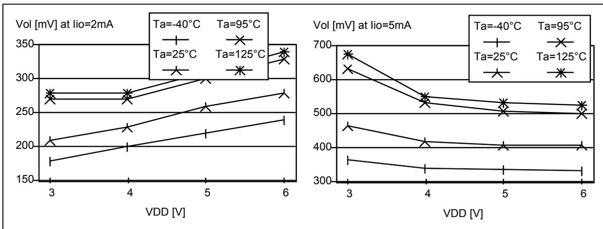
Figure 67. Typical  $V_{OL}$  vs  $V_{DD}$  (high-sink I/Os)
