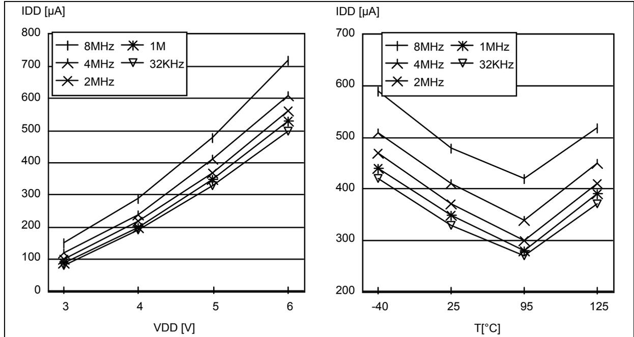
Figure 45. Typical  $I_{DD}$  in WAIT vs  $f_{CPU}$  and Temperature for OTP devices with option bytes programmed to 00H
