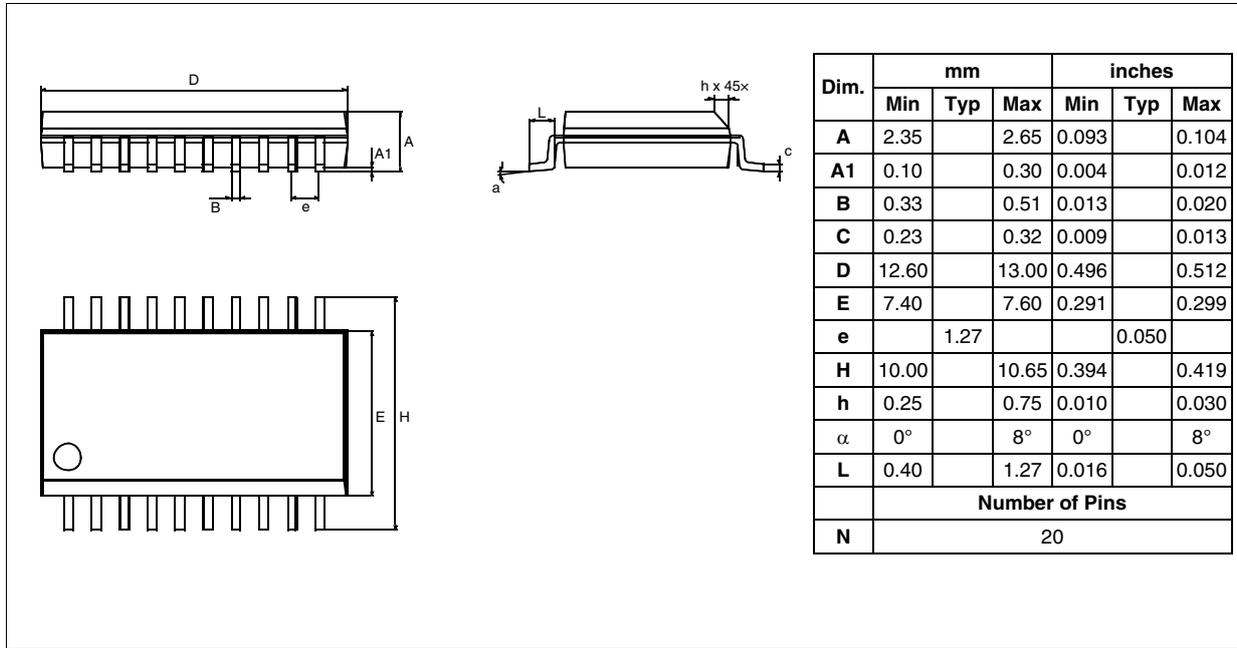
Figure 77. 20-Pin Plastic Shrink Small Outline Package
