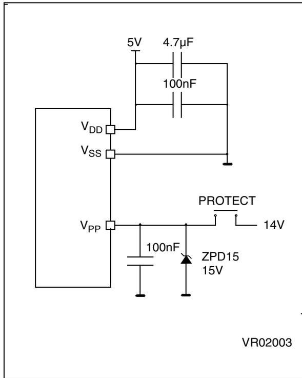
**Note:** ZPD15 is used for overvoltage protection
