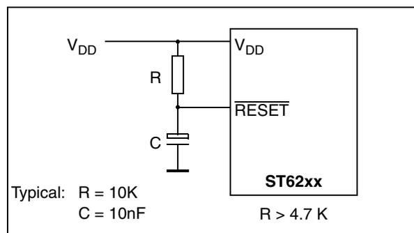
Figure 16. Reset Processing
