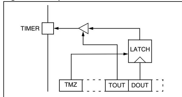
**Figure 33. Output Mode Operation**
