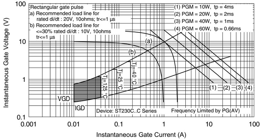
Fig. 11 - Gate Characteristics
