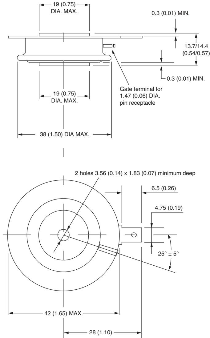
Quote between upper and lower pole pieces has to be considered after application of mounting force (see thermal and mechanical specification)
