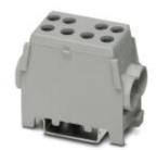
Trunk line branch terminal, Connection method: Screw connection, Screw connection, Number of connections: 4, Number of positions: 1, Cross section: 10 mm² - 35 mm², AWG: 8 - 2, Width: 27 mm, Color: gray, Mounting type: NS 35/7,5, NS 35/15
