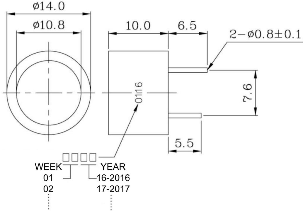
Note 1. Part is designed as a sealed transducer to protect inner structure.
