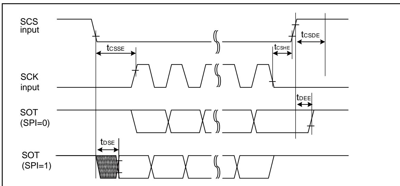
**When Using High-speed Synchronous Serial Chip Select (SPI = 1, SCINV = 0, MS=0, CSLVL=0)**
