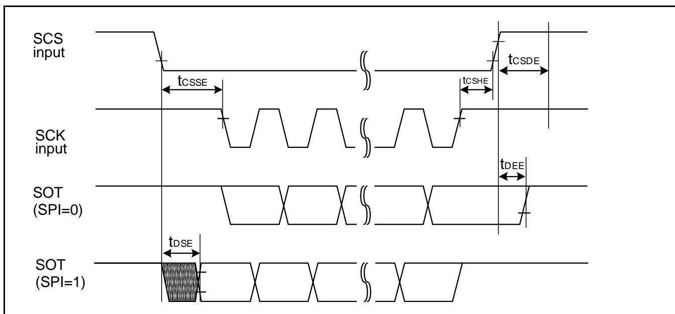
**When Using High-speed Synchronous Serial Chip Select (SPI = 1, SCINV = 1, MS=0, CSLVL=1)**
