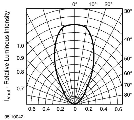
Fig. 7 - Relative Luminous Intensity vs. Angular Displacement
