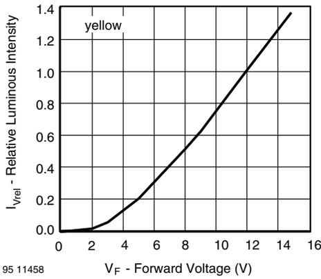
Fig. 4 - Relative Luminous Intensity vs. Forward Voltage
