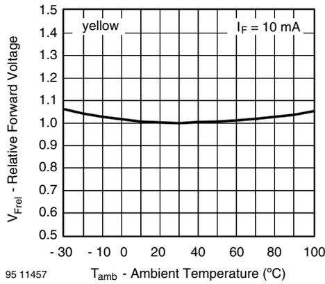
Fig. 3 - Relative Forward Voltage vs. Ambient Temperature
