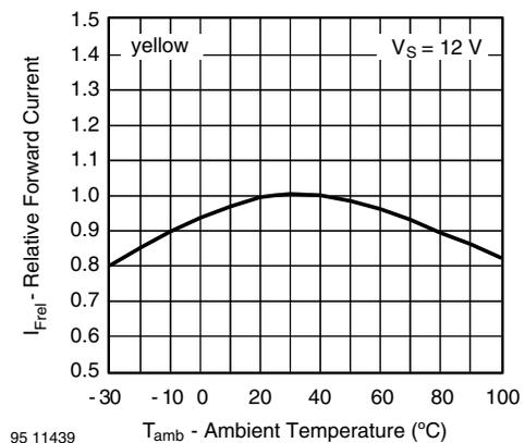
Fig. 2 - Relative Forward Current vs. Ambient Temperature
