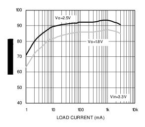
Figure 3. Efficiency vs Load Current (Burst Mode, 550kHz)
