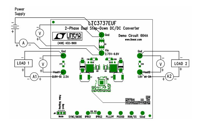
Figure 1. Proper Measurement Equipment Setup
