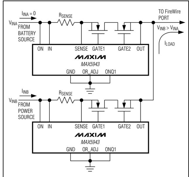
Figure 5. MAX5943 ORing Controller Rerouting Load Current
