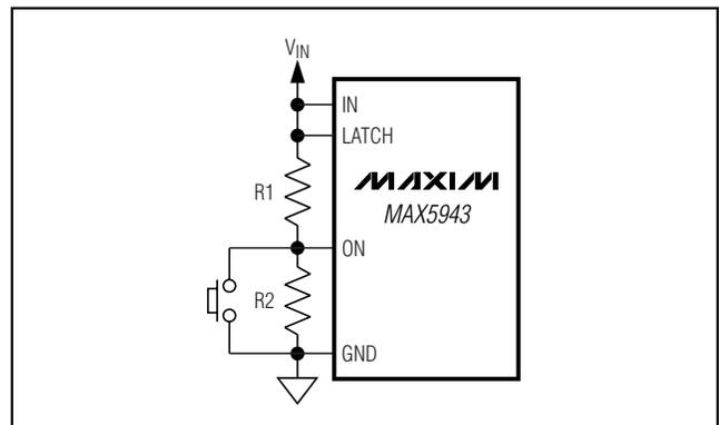
Figure 9. Resetting MAX5943 After a Latched Fault Condition
