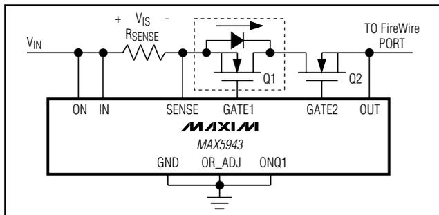
Figure 4. Q1 Current Path During Initial Startup
