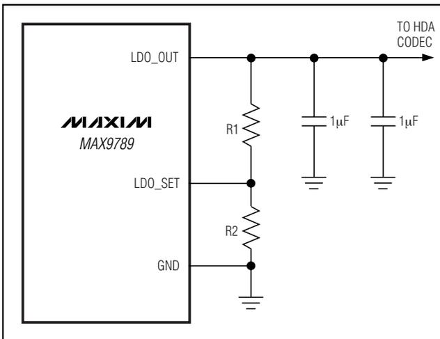
Figure 1. Adjustable Output Using External Feedback Resistors.
