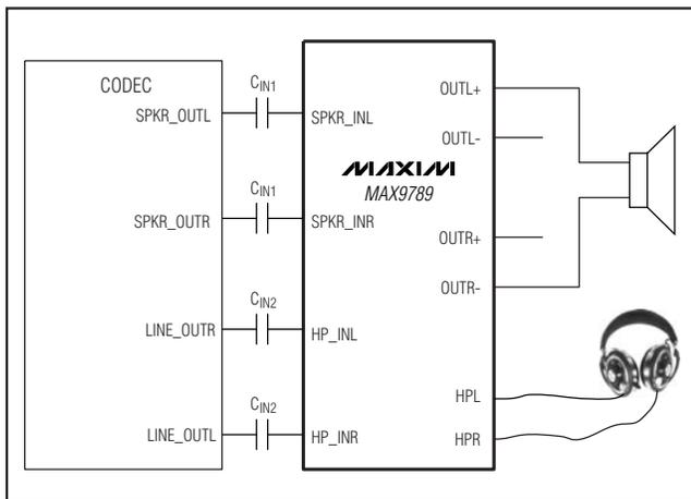
Figure 6. Mono Signal Output Configuration for MAX9789
