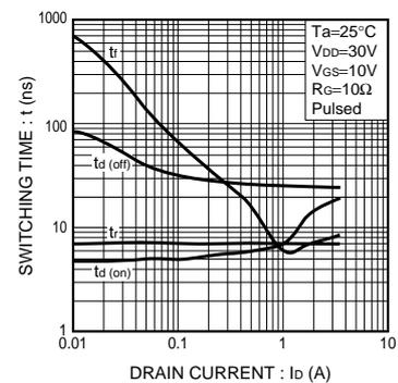
Fig.9 Switching Characteristics
