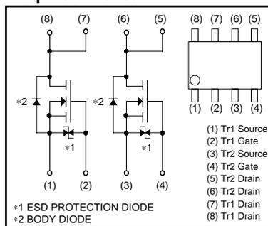
\*1 A protection diode is included between the gate and the source terminals to protect the diode against static electricity when the product is in use. Use the protection circuit when the fixed voltages are exceeded.
