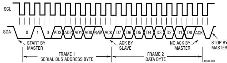
Figure 9. Reading the Interrupt Register (Short Form)
