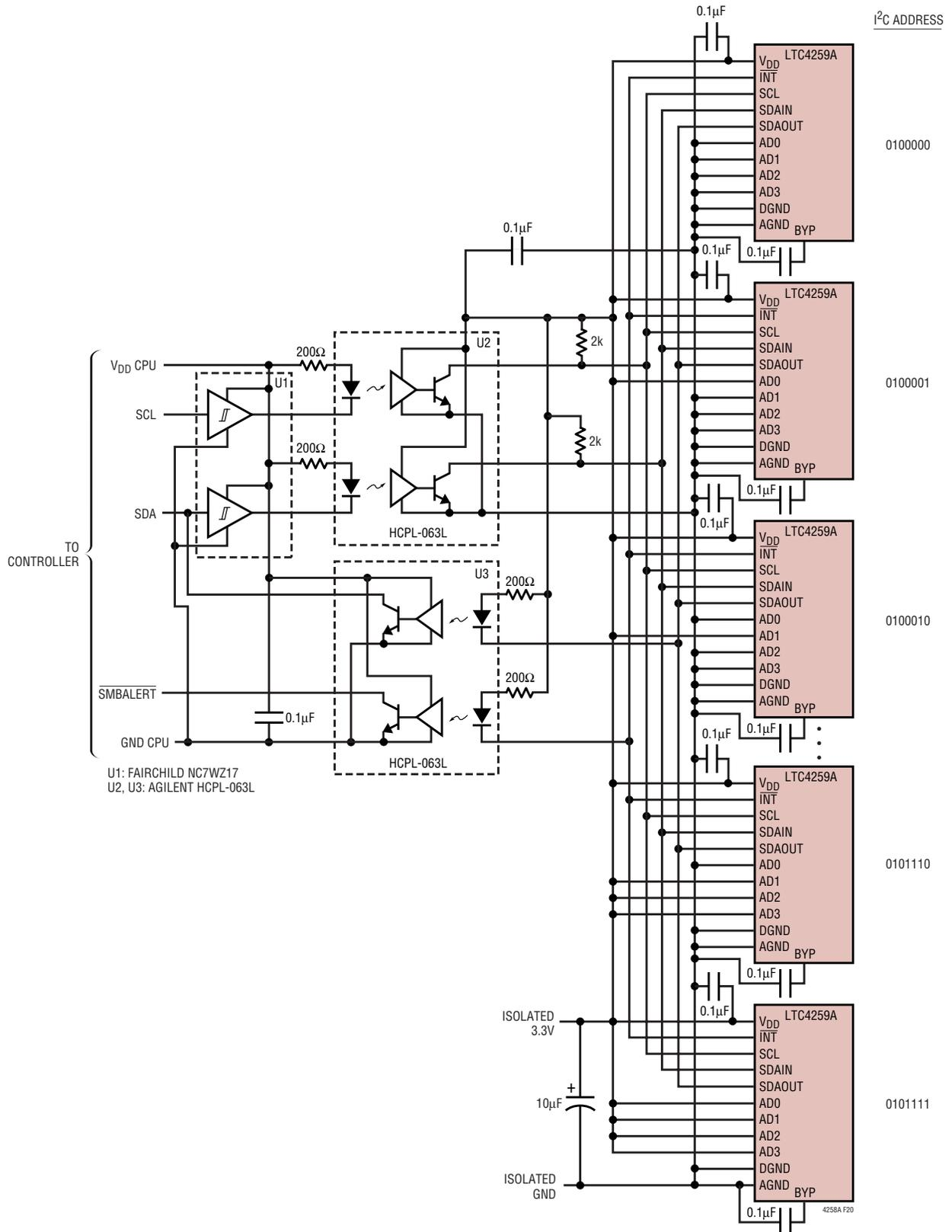
Figure 20. Optoisolating the I<sup>2</sup>C Bus
