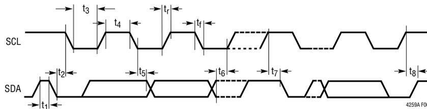
Figure 6. I<sup>2</sup>C Interface Timing
