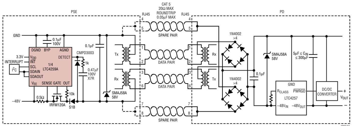
Figure 11. Power over Ethernet System Diagram
