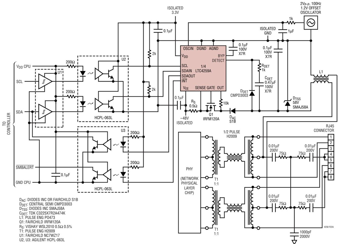
Figure 22. One Complete Isolated Powered Ethernet Port
