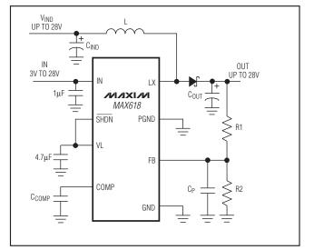
Figure 4. Dual-Supply Operation ( $V_{IN} = 3V$  to 28V)
