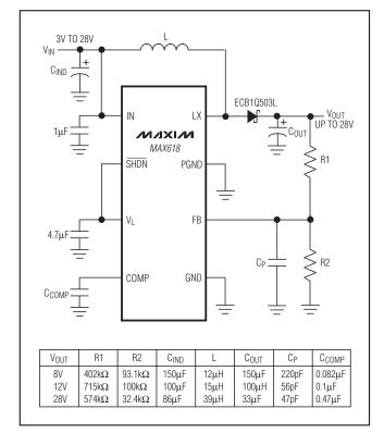
Figure 1. Single-Supply Operation
