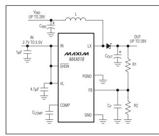
Figure 3. Dual-Supply Operation ( $V_{IN} = 2.7V$  to 5.5V)
