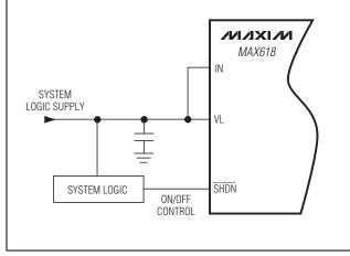
Figure 6. Adding On/Off Control to Circuit of Figure 3
