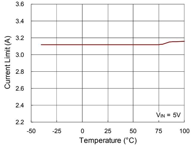
**Over Current Trip Threshold vs. Temperature**
