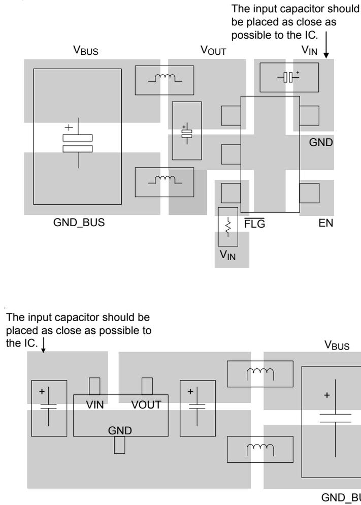
Figure 2. PCB Layout Guide
