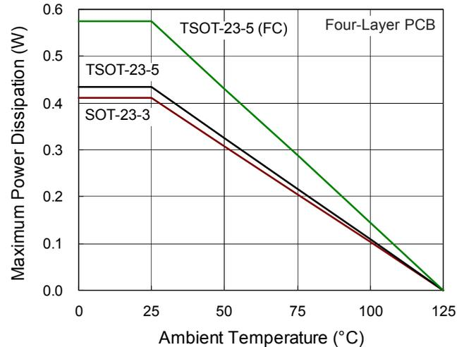
Figure 1. Derating Curve of Maximum Power Dissipation
