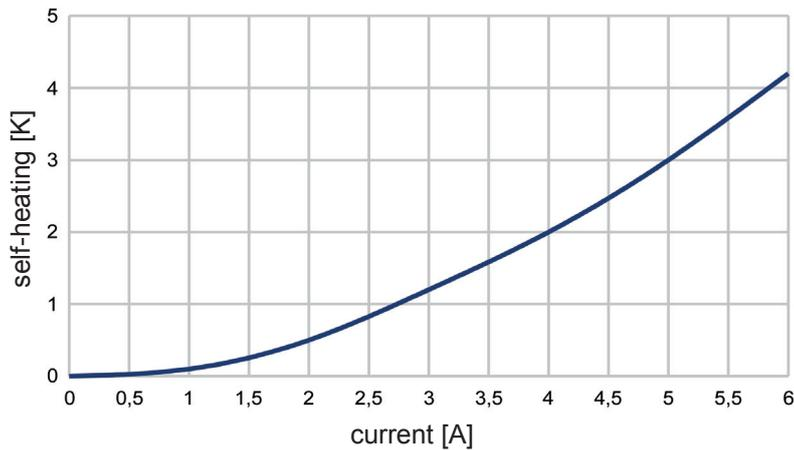
The characteristic curve in the diagram is measured with a thermal control without any insulation in an oil bath.
