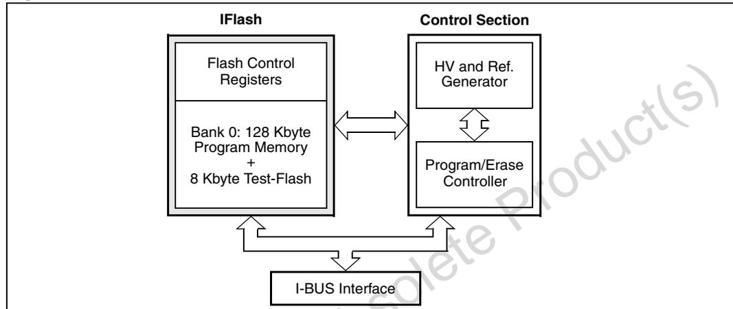
The programming operations of the Flash are managed by an embedded Flash Program/Erase Controller (FPEC). The High Voltages needed for Program/Erase operations are internally generated.
