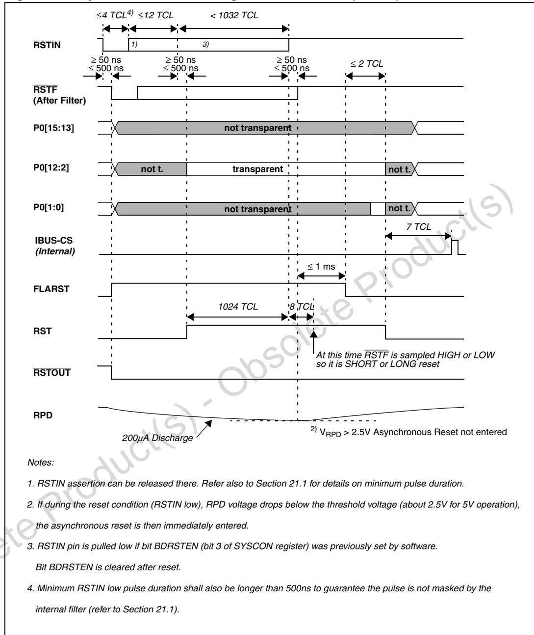
Figure 22. Synchronous short / long hardware reset ( $\overline{EA} = 0$ )
